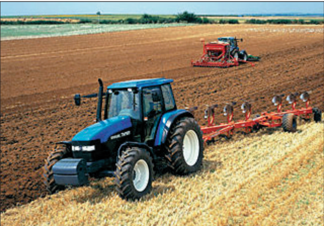
Driving heavy tractors on the subsoil during ploughing and harvesting is a major cause of subsoil compaction. The picture clearly shows how the wheels on one side of the tractor are driven in the plough furrow and press directly on the subsoil (JHVEDA).
