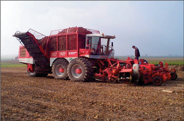
Areas degraded by soil compaction are increasing because wheel loads in agriculture are still increasing. Twenty years ago wheel loads of 50 kN (5000 kg) were considered very high. Nowadays wheel loads of up to 130 kN are used during the harvesting of sugar beet. Modern self-propelled slurry tankers with injection equipment with wheel loads of 90 – 120 kN are used in early spring on wet soils. Large tyres with an inflation pressure of about 200 kPa are needed to carry such high wheel loads. Even on moderate strong soil, compaction of up to 80 cm below the surface have been measured under such loads. The result is that the soil is increasingly compacted to ever-greater depth. The conclusion is that European soil is more threatened than ever (JHVEDA).
